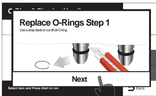
Use a sharp blade to cut off the old O-Ring according to the step showing on the screen and then press NEXT after finishing the step.
