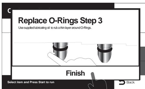
Spread lubricating oil on the O-Ring and press Finish.
