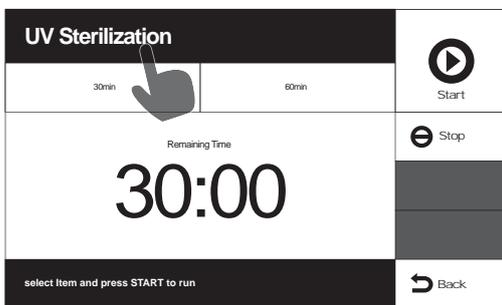
You can select thirty minutes process or sixty minutes process in the UV Sterilization menu and then press START to begin sterilization. During the process, the touch screen will show the remaining time for the sterilization and then show the completing screen after the sterilization is completed.
